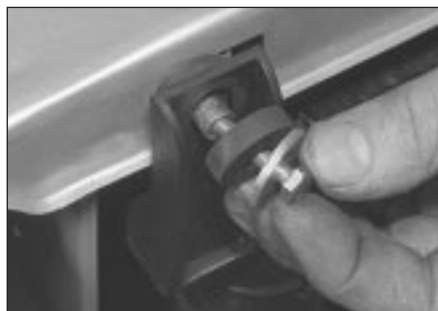
7.6a Radiator securing bolt, insulator and washer
