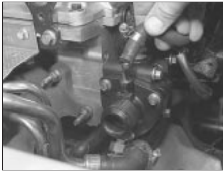
4.8 Disconnect the coolant hoses from the water outlet on a Zetec engine
