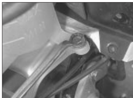
7.22a Remove the single bolt retaining the expansion tank . . .
