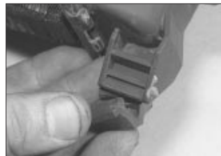
7.6b Rubber insulator on radiator locating lug
