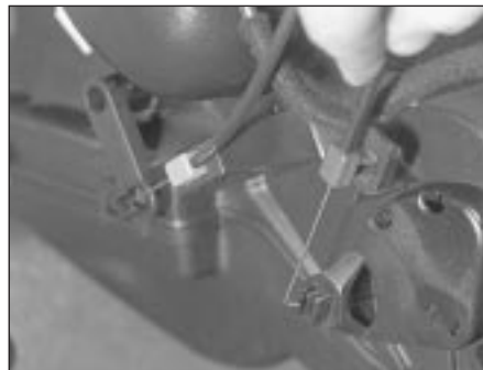
11.5 Disengaging heater control cable from its flap operating mechanism on the heater casing
